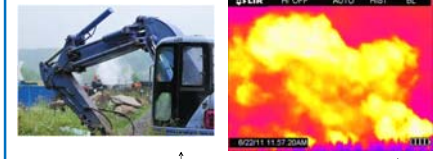
What the naked eyes sees ↑ What IR photography sees (massive methane release)
