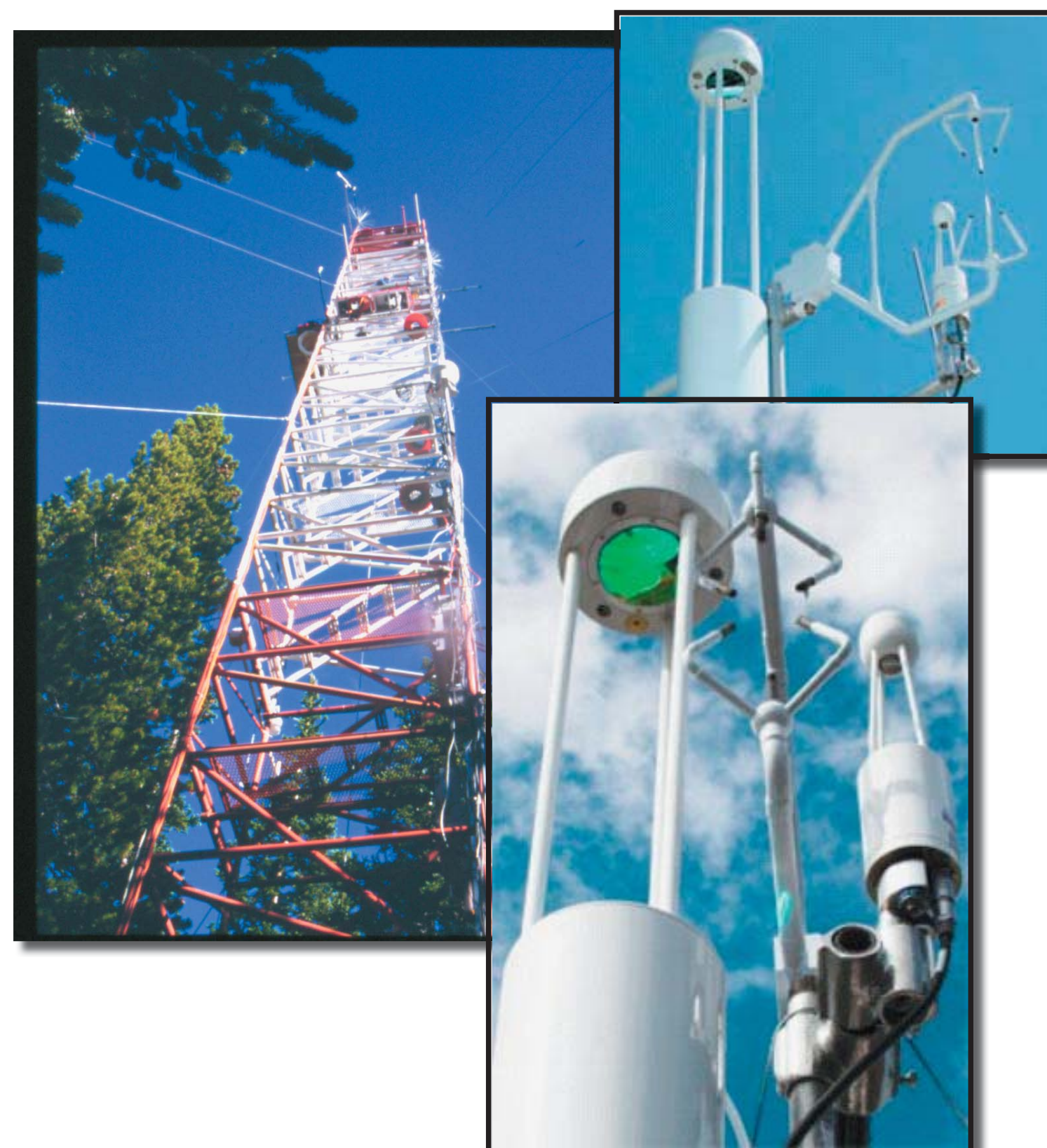
The eddy covariance method [above; source: Burba and Anderson (2005)] takes advantage of the way air behaves near the surface of the Earth. The surface is rough and slows down the air and causes it to rotate or 'eddy'. Simultaneous measurements of the direction (up or down) the air is moving and the concentration of a gas of interest (e.g., carbon dioxide, methane, etc.) can be used to calculate the net movement of the gas. For the measurement to be robust, the measurements must be made at very high rates (> 10 measurements per second). Therefore, in the case of methane we measure the wind speed and direction using sound and the concentration of methane using the absorption spectrum of a precision laser [below]
