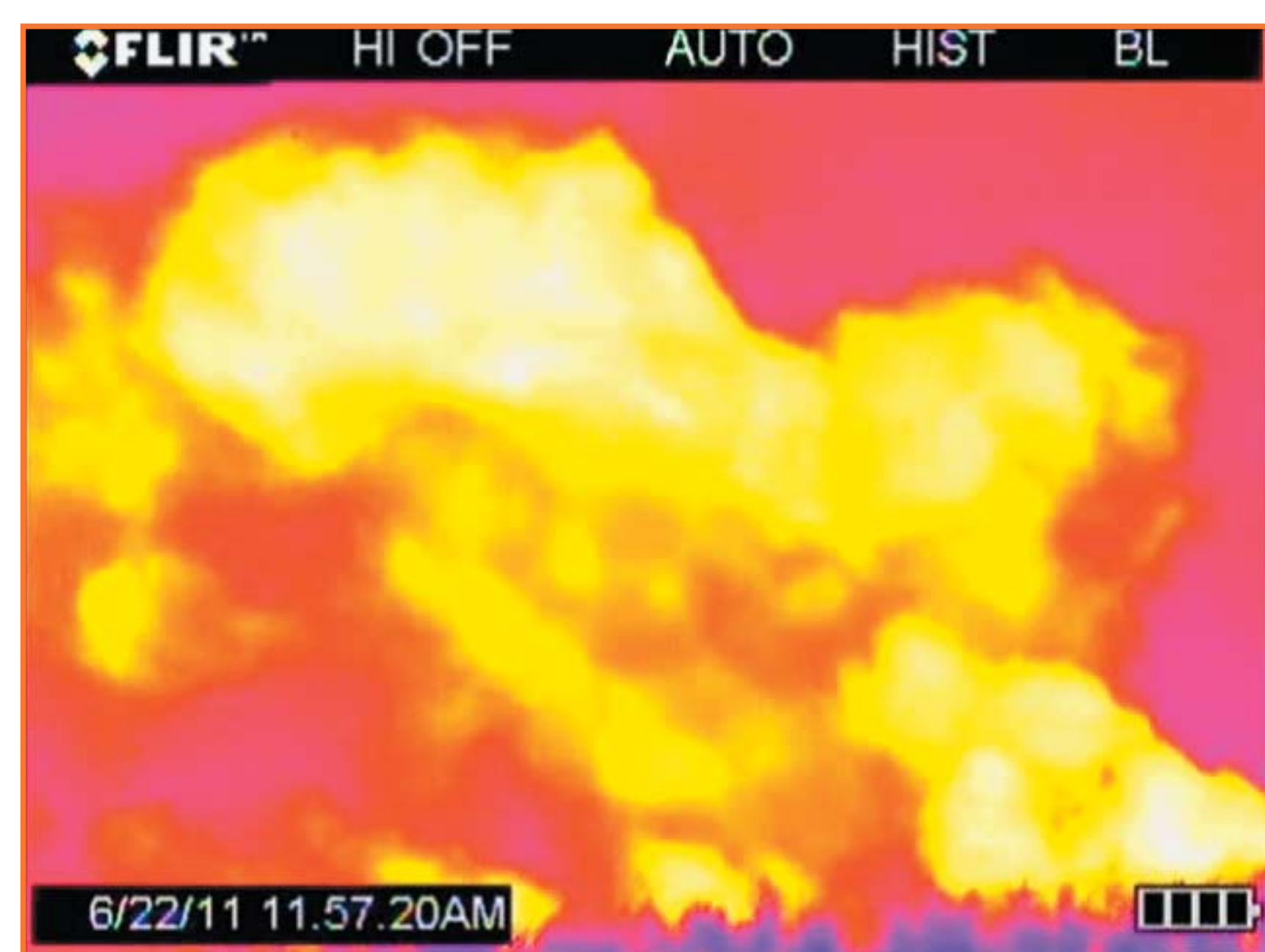
Natural gas is invisible to the naked eye, so infrared cameras are often used to detect leaks in the system; here an infrared video camera captures the completion vent from Marcellus gas well. Still taken from video footage courtesy Frank Finan.
